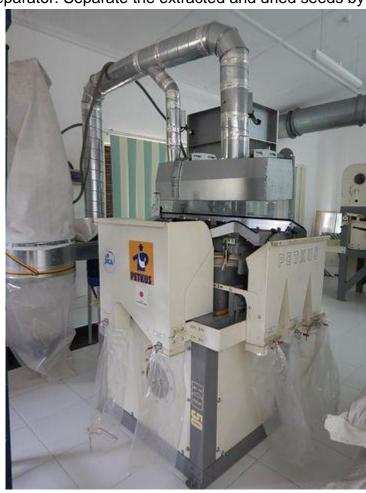
Color Soter: Separate the extracted seeds by the colour
