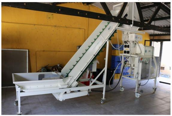
Gravity Separator: Separate the extracted and dried seeds by the weight
